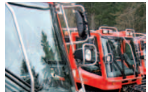
The brush-guards protect the windscreen and the headlights from whipping branches.
